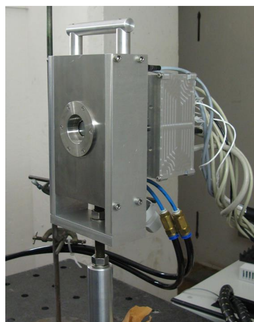
The SLcam or Color X-ray Camera, a prototype hyperspectral X-ray detector
